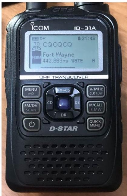
ICOM ID-31A D-STAR/FM UHF handheld transceiver. UHF only. Up to 5 watts output. Built in GPS receiver. Programmed for
