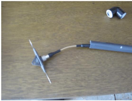
I attached my RF Choke Balun to my dipole center. (I don't use a traditional W2AU type balun with the fear that 1500 watts could fry it! The Coax Choke Balun uses 60 small common mode chokes around coax.) Use super glue or PVC cement to attach the dipole center to the 12 inch pipe.
