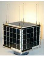
51 is a popular Amateur Radio satellite that often functions as a crossband FM repeater, relaying brief conversations over hundreds of miles. Formosat 3D is part of a constellation of six remote sensing microsatellites that collect atmospheric data for weather prediction and for ionosphere, climate and gravity research. Both orbit at an altitude of approximately 500 miles.
