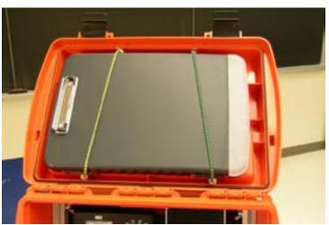
operating aids such as operator's license, message forms, technical guides, and maybe a city/county map. I found a plastic note keeper that can double as a clipboard at Office Depot. It fits the lid ideally and doesn't interfere with the IC-208H front panel when the lid is closed.
